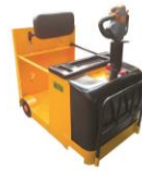
TOW TRACTOR MEL 3310 – 40/RTT. Capacity – 1000 – 4000 kg.
